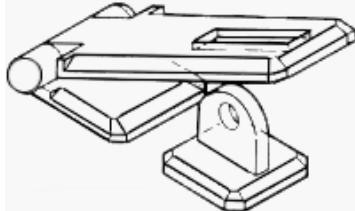
**Reversible Locking System:** Bottom section of hasp is reversible for either corner or flatmounting. Predetermine assembly before inserting pin completely!
